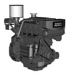
4-cylinder, 4-stroke, direct-injected, turbo-charged, and aftercooled (TA version) marine diesel engine. Bore x Stroke (mm): 108 x 130 Displacement (I): 4.76
