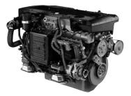
4-cylinder, 4-stroke, direct-injected turbo-charged, and aftercooled marine diesel engine. Bore x Stroke (mm): 103 x 110 Displacement (I): 3.67 6-cylinder, 4-stroke, direct-injected turbo-charged, and aftercooled marine diesel engine. Bore x Stroke (mm): 103 x 110 Displacement (I): 5.5
